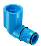
Designed for use with female acme thread O-ring seal style rotors. Provides faster installation and positive O-ring seal. Reduces the risk of overtightening and eliminates the need for thread sealants. Available as an individual component.
