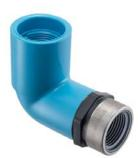
Designed for use where overtightening of threads is a problem. This unique precompression design compensates for expansion forces generated from tapered pipe thread joint makeup. Radial stress is reduced in normal installations and contained in severe overtightening situations. Available as an individual component.
