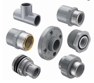
SPEARS® Schedule 80 CPVC pipe and fitting designs combine years of proven experience with computer generated stress analysis to yield the optimum physical structure and performance for each fitting. Material reinforcement is uniformly placed in stress concentration areas for substantially improved pressure handling capability. Resulting products are subjected to numerous verification tests to assure the very best CPVC piping products available.
