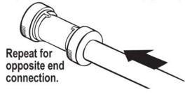
WARNING: DO NOT INSERT FINGERS. ENSURE THAT PIPE AND FITTINGS ARE FREE OF DIRT AND DEBRIS PRIOR TO INSTALLATION.
