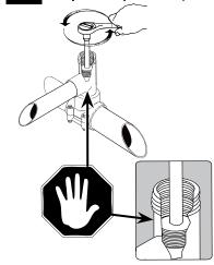
STEP 6 Back-off Cutter to Top to Open Flow
