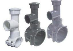
Specially designed tapping saddle allows pipe branch connection to pressurized "Hot" lines without system shut-down. Available in PVC White, Gray or CPVC Gray configurations.
