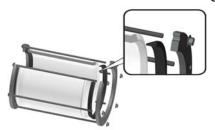
Bolt Tightening Sequence Recommended Torque to Seal: 12-15 ft-lb
