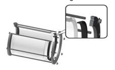
6",8"-4 bolt 10" -5 bolt 12" -6 bolt 15" -7 bolt
