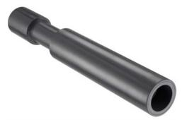
Linear expansion and contraction from temperature fluctuations can be a major problem in thermoplastic piping systems. Forces left uncontrolled can literally tear systems apart. Spears® Expansion Joint allows a telescoping movement of an inner pipe within a firmly mounted outer tube to eliminate such damage. Available for CPVC 1/2" through 12" and PVC 1/2" through 14" IPS piping systems in 6" or 12" maximum travel lengths. Custom produced for virtually any pipe diameter.
