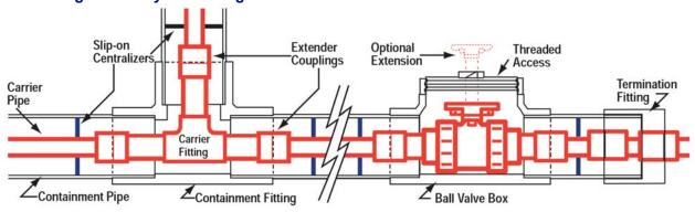
Carrier fittings are equipped with special extender couplings for connection to carrier pipe. Simple, slip-on centralizer brackets used on the carrier pipe support this assembly inside the containment pipe. This design allows the carrier fitting to "float" within the containment fitting, allowing ease of movement for installation while reducing problems associated with thermal expansion and contraction during operation.
